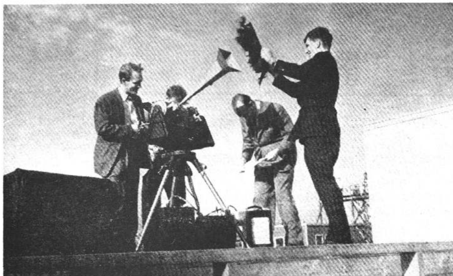
Fig. 1. Early 1.5 cm microwave radiometer surrounded by (left to right) E. Beringer, R. Kyhl, A. Vane, and R. H. Dicke. Dicke is shaking the "shaggy dog" - a piece of absorbing material used as a calibration source.
