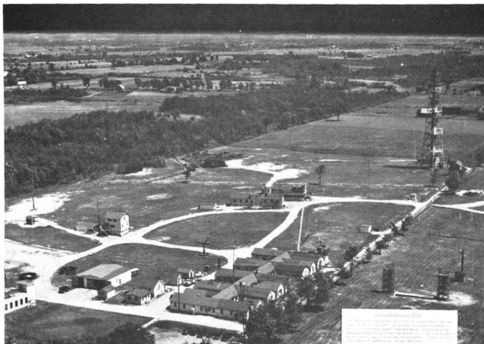
Fig. 4. Aerial view of the Radio Field Station of the National Research Council of Canada outside of Ottawa, circa 1949. The 10.7 cm partial solar eclipse observations were made from the roof of the building in the lower left. The 200 ft tower used for the 150 cm radars is on far right.
